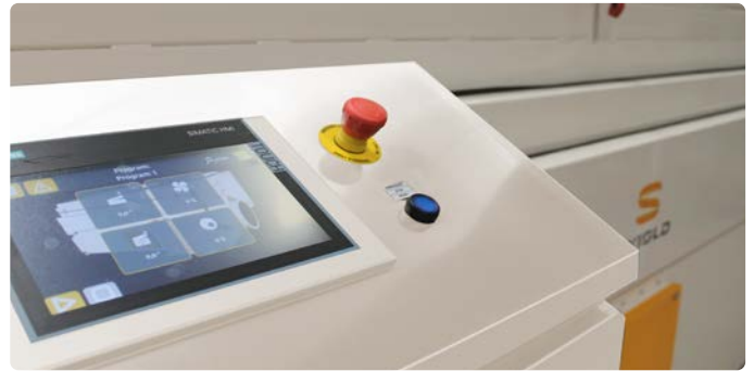
Control based on Siemens PLC
